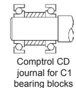
For applications requiring thermal expansion of the screw and/or higher speeds, a Comptrol Type CD journal is typically used on one end of the screw. The bearing block used with the Type CD journal will not share the load equally.
