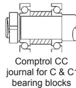
**Type C & C1** bearing blocks have spaced, bidirectional angular contact bearings to provide the rigid end support needed to achieve higher speeds and increased stiffness of the overall ballscrew assembly.
