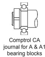
**Type A & A1** bearing blocks use a single sealed radial ball bearing to provide simple radial end support. They are primarily used to prevent whipping and radial deflection of the ballscrew centerline in light load applications where axial positioning accuracy is not critical.
