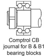
**Type B & B1** bearing blocks feature duplex, bidirectional angular contact bearings to control axial movement of the screw. They also provide higher axial thrust and radial load capacities than "A" type bearing blocks.
