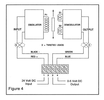
With Comptrol LVDT's the input and output circuits are electrically isolated from each other and from the mechanical structure of the loadcell. Thus, they may be used in "floating ground" or "ground return" systems.
