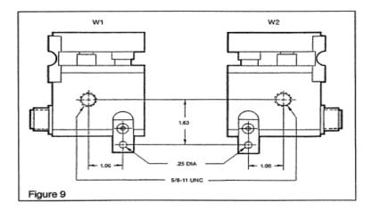
A locating tab prevents the Tensioncell from rotating and secures it in a permanent location. It also provides a means of repeating rotatory position when the Tensioncell needs replacement. (See Figure 9)
