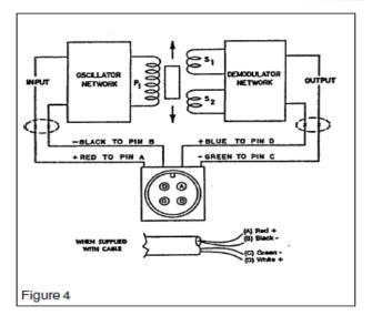
With Comptrol LVDTs, the input and output circuits are electrically isolated from each other and from the mechanical structure of the Tensioncells. Thus, they may be used in "floating ground" or "ground return" systems. This eliminates the need for extra circuit boards which are required for most strain gage loadcells.
