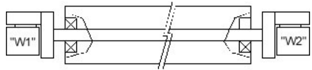
TYPE B - Bearing in Roll - Nonrotating Shaft Self aligning Shaft Mounts in Tensioncells
