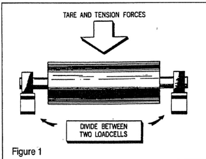
For our discussion here, deflection of the Load Plate the Base Block is defined as the "Compression Mode", while the opposite is defined as the "Tension Mode". Tensioncells are designed to operate equally well in either mode.
