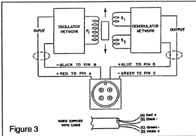
In standard applications, where two Tensioncells are used, the inputs may be connected in parallel allowing the Tensioncells to be excited from the same power supply. The LVDT outputs are then summed to obtain a signal representing the strip tension and tare loads distributed across the roll
